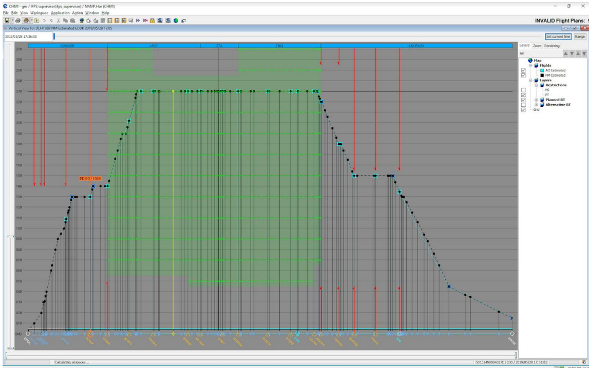
Figure 11: Example 4 - Vertical profile for AU Trajectory with PTR implementation and IFPUV trajectory
